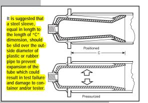
And when the test is finished, the SWEL-PLUG Pressure Tester can be removed with a minimum of effort because its grip to the pipe walls slackens automatically as internal pressure is relieved.
